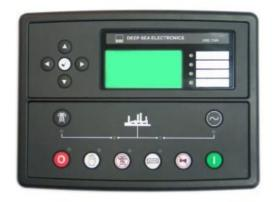
The DSE7320 is an Auto Start & Auto Mains (Utility) Failure Control Module suitable for a wide variety of single, diesel or gas, gen-set applications. It monitors speed, frequency, voltage, current, oil pressure, coolant temperature and fuel level, and the modules will display warnings, shutdown and engine status information on the backlit LCD screen and illuminated LED.
